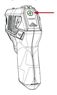
An orange LED indicates a "low" battery. In some conditions, especially low temperature (-4 °F/-20 °C) the LED may display orange even if the battery has sufficient charge left.
